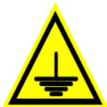
Ensure that the grounding cable, which is already connected to the control, is connected to the relevant and marked ground wire end on the irradiation chamber before the UV system is put into use. Check whether the irradiation chamber has a good electrical connection with the ground contact in the plug.
