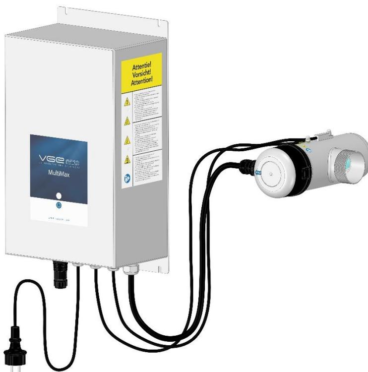
The heart of the UV system is the irradiation chamber which is provided with one medium-pressure UV lamp which combines a compact design with a high lamp power. An inline design of the irradiation chamber has been chosen with a UV lamp placed perpendicular to the direction of the flow in order to obtain good irradiation of the water in combination with a very low hydraulic pressure loss.
