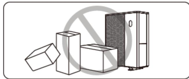
1.4.4. Do not put anything into the inlet or outlet, and do not remove the fan cover and the running fan to avoid injury.
