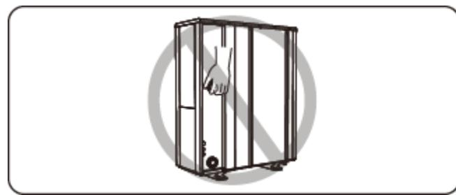
1.4.3. Don't put obstacles before the air inlet and outlet of the heat pump.
